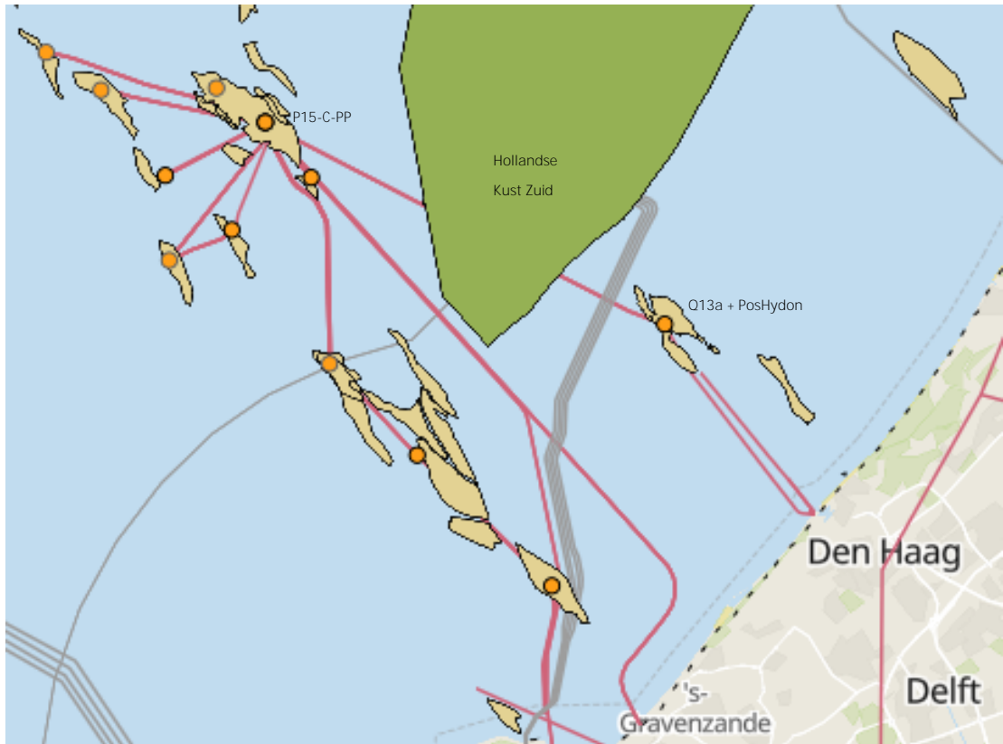
Figure 36. Platforms connected to pipeline DPL-15D1 (red), operated by TAQA.
