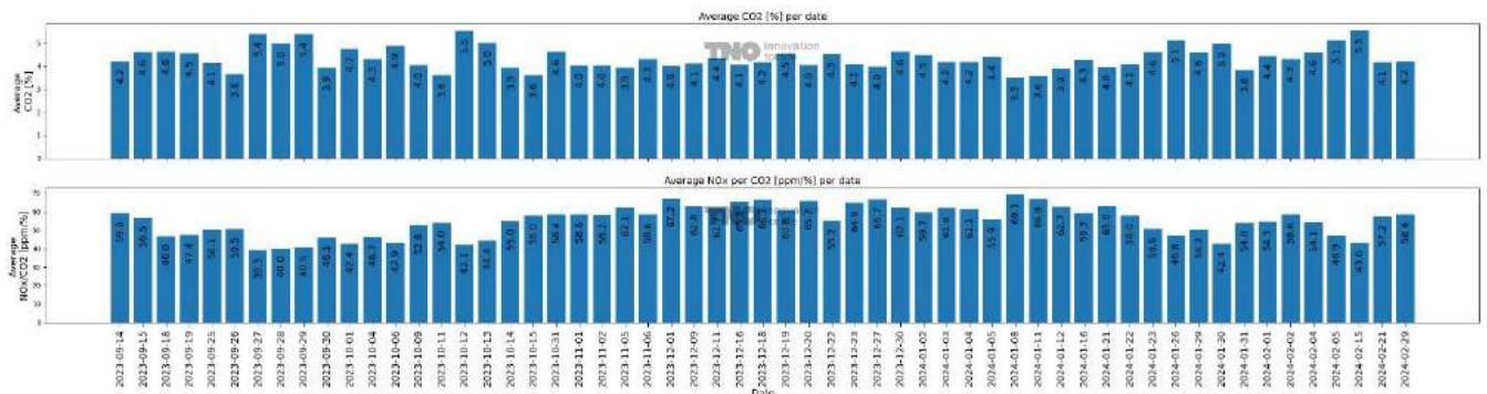
Figure 4.3: CO 2 and NO x /CO 2 emissions per active calendar day for the TH_300_STAV.
