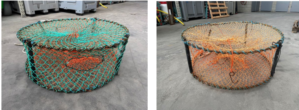
Figure 2.7 – Cuttlefish pot with fluorescent netting (left) and cuttlefish pot with original netting (right). Photo's: Wageningen Marine Research.
