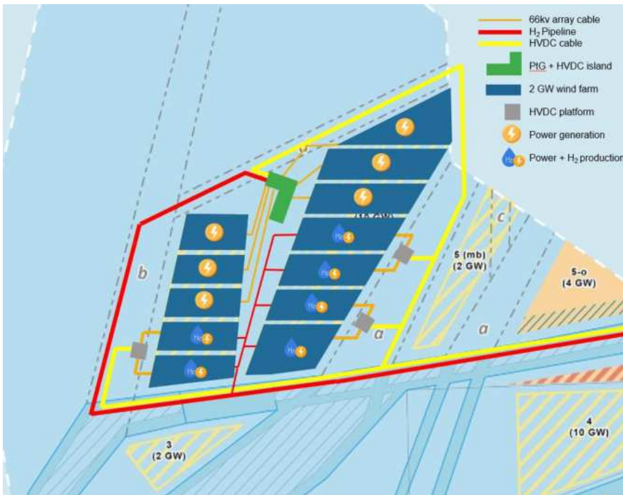
Figure 6.6: Illustrative Layout of Hybrid-based Energy Hub.
