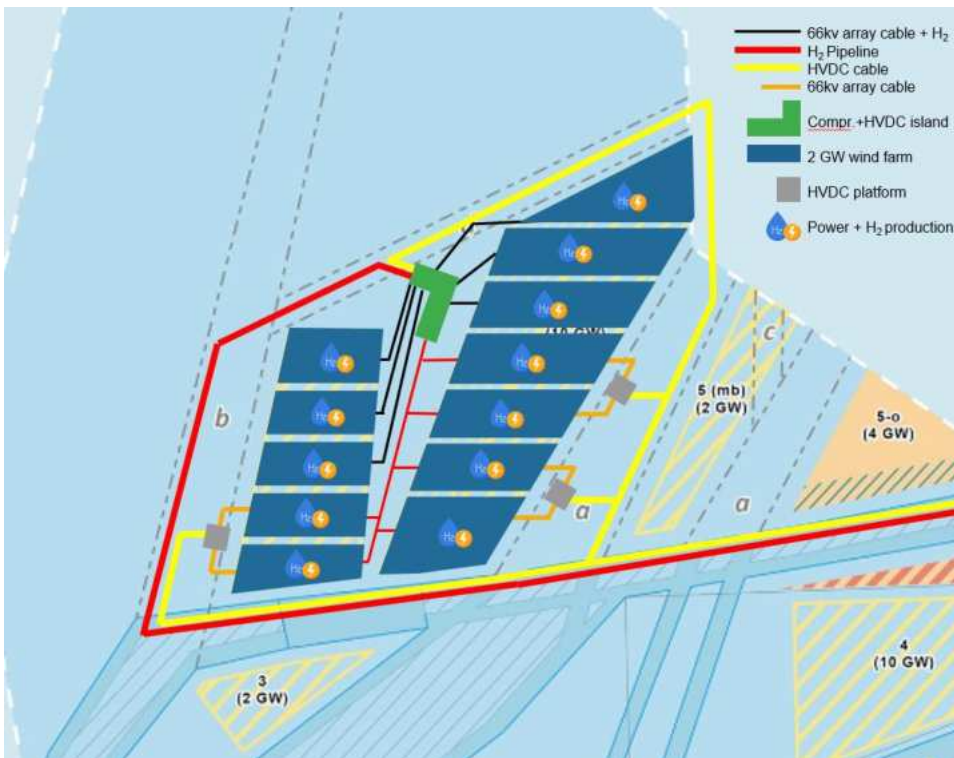
Figure 6.22: Illustrative Layout of Concept 3 – Platform-based Hub but with Centralised Compression/HVDC on an Island.
