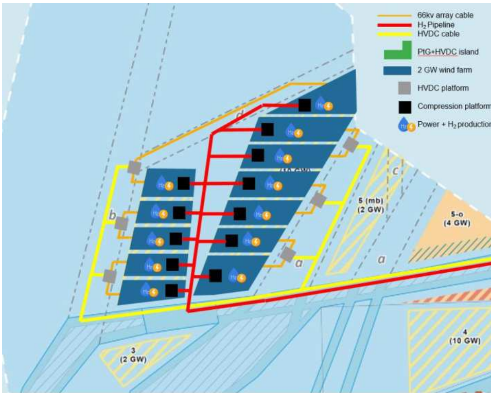
Figure 3.6: Illustrative Layout of Concept 2b – Platform-based Hub including Decentralised Compression
