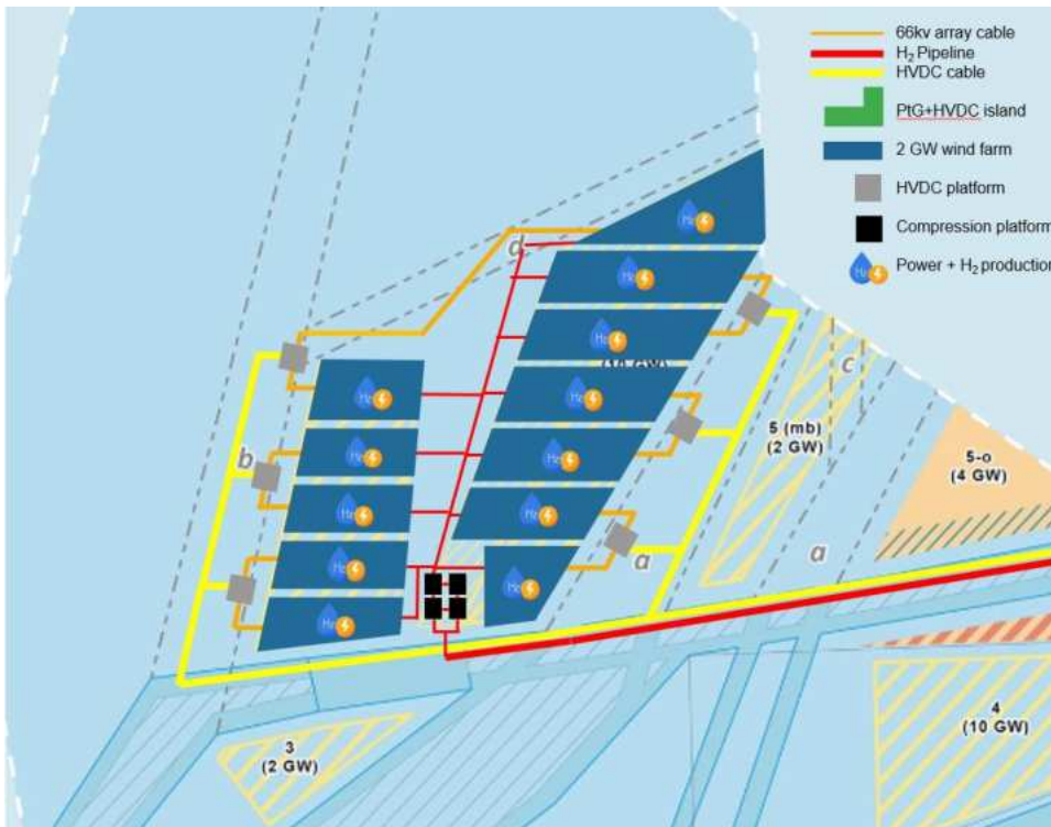
Figure 6.20: Illustrative Layout of Concept 2a – Platform-based Hub including Centralised Compression
