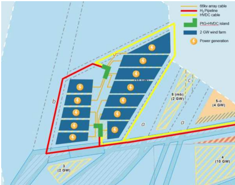
Figure 6.1: Illustrative Layout of Island-based Energy Hub (concept 1).
