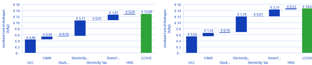
Figure 4.3: Breakdown of LCOH 2 for cases with 5,300 (left) and 4,300 (right) FLH, respectively.
