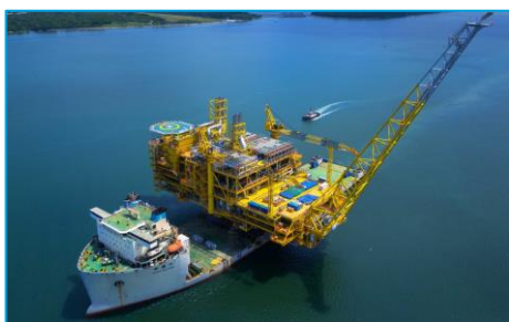
Figure 2 - Example of heavy lift ship
