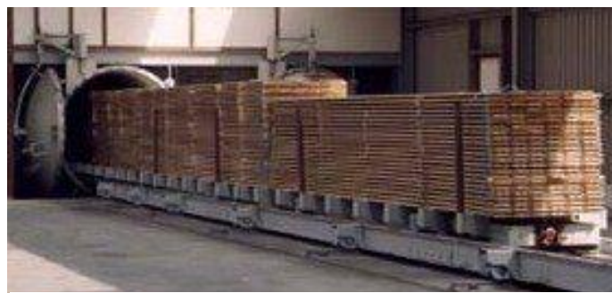
Figure 5 - Wood preservation in an autoclave 13
