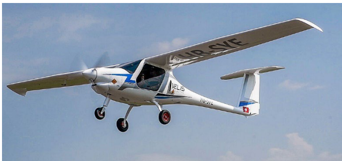
Pipistrel Velis Electric: operational electric 2-seater
