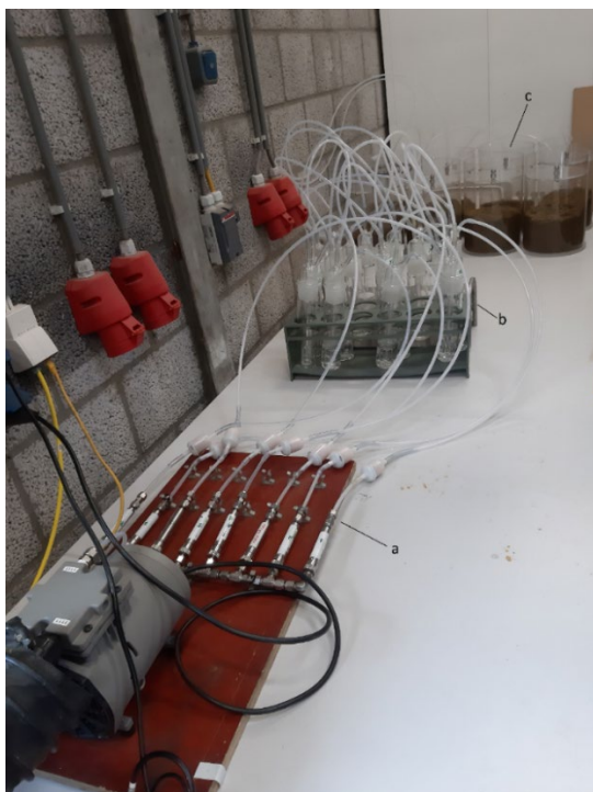
Figure 3 Impinger set-up for measuring \text{NH}_3 emission from manure a) vacuum unit, b) impinger unit and c) vessel unit
