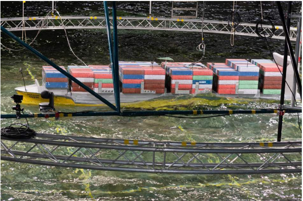
Photo 14 Test 33327_01OB_04_004_009_01: \mu = 270 deg – H_s = 4.5 m – T_p = 8.5 s
