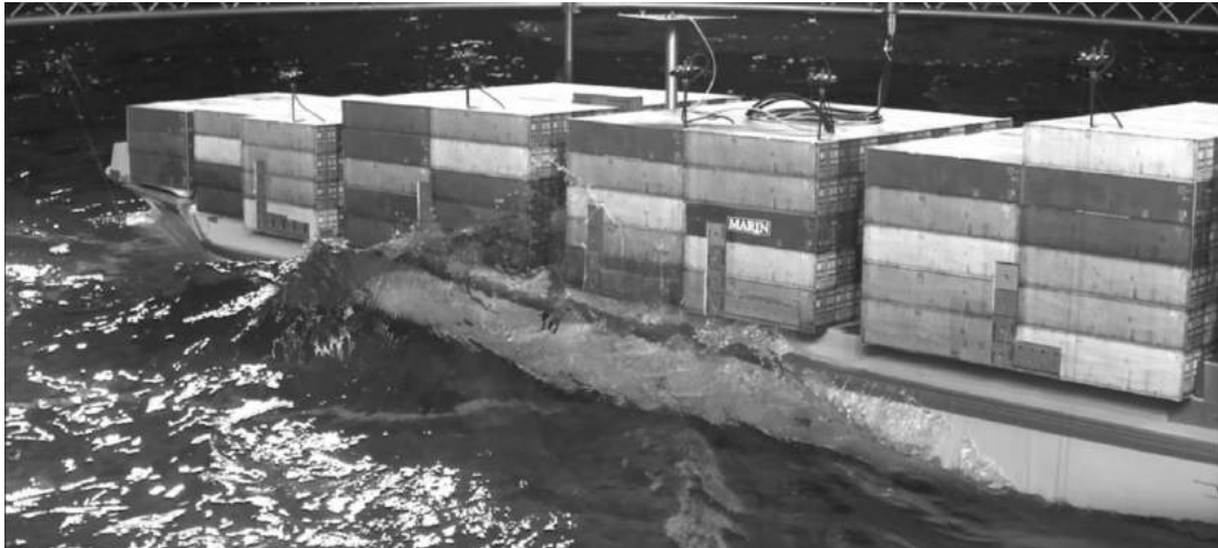
Figure 3-17: Green water load from in stern-quartering waves
