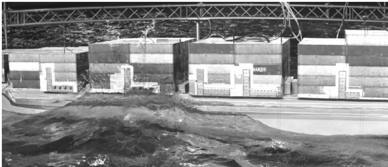
Figure 3-32: Takes of the largest transverse and vertical impact from green water taken shortly after each other, configuration 2, H_s = 4.5 m, T_p = 8.5 s, heading 270 deg
