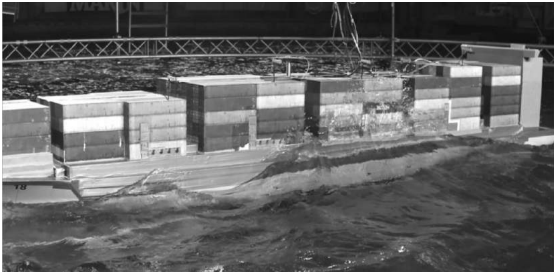
Figure 3-16: Green water load from steep, breaking beam waves
