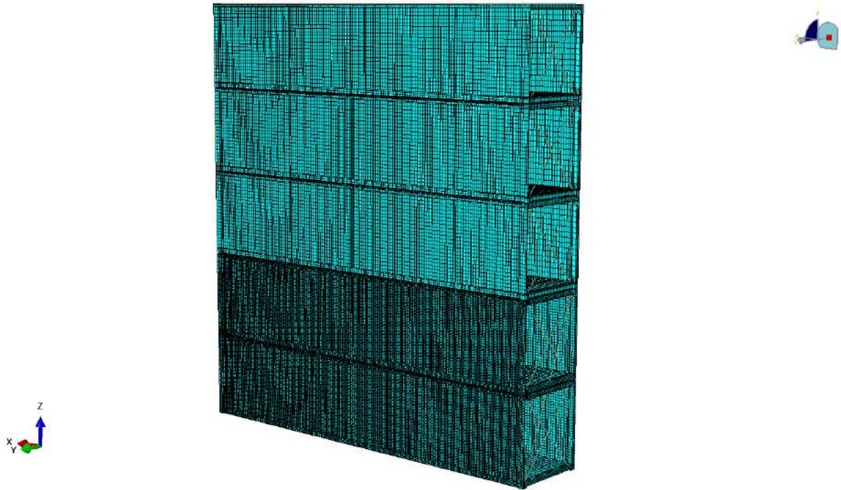
Figure 5-2: FEM mesh of the container stack
