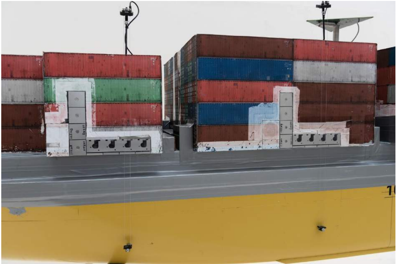
Photo 12 Details of the force panels
