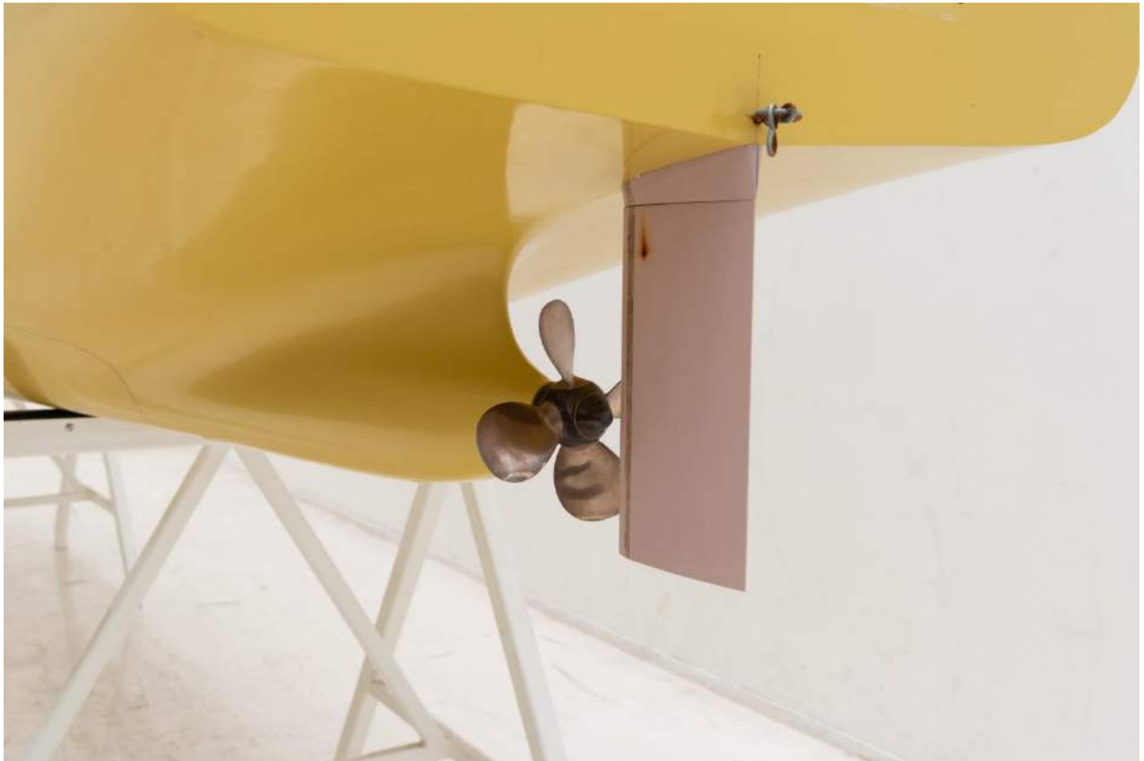
Photo 6 Details of the rudders and propellers
