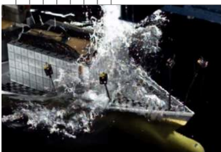
Extreme event matching applied to determine local and global wave impact loading on the breakwater of a container vessel (courtesy of the CRS working group green water).
