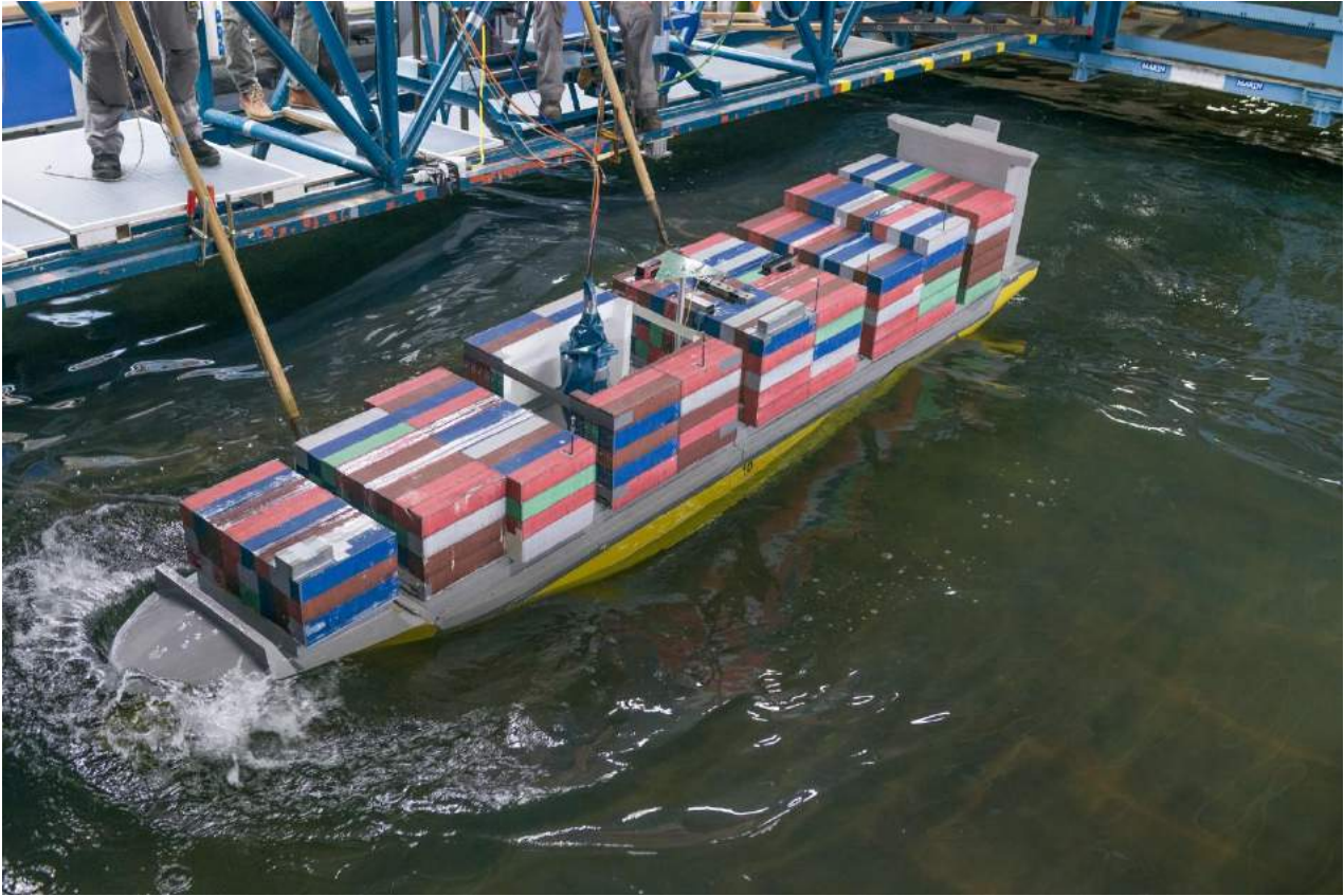
Photo 16 Test 33327_02BT_04_001: \mu = 180 \text{ deg} – H_s = 6.0 \text{ m} – T_p = 11.8 \text{ s} – V_s = 4 \text{ kn}
