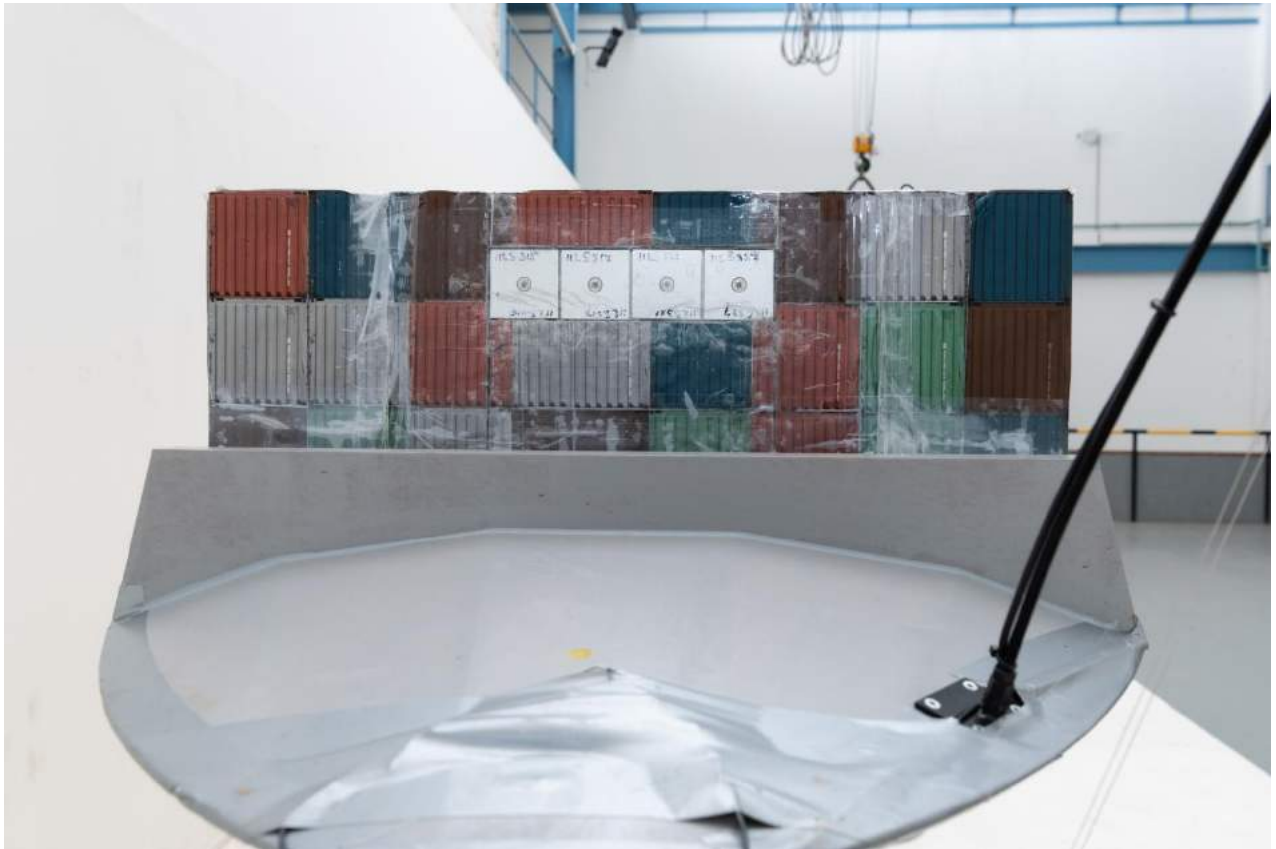
Photo 10 Details of the force panels
