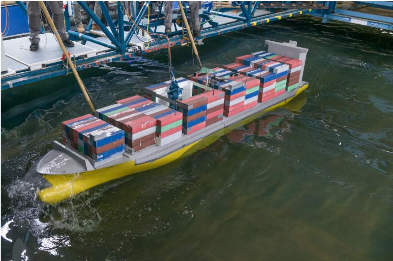
Photo 16 Test 33327_02BT_04_001: \mu = 180 \text{ deg} – H_s = 6.0 \text{ m} – T_p = 11.8 \text{ s} – V_s = 4 \text{ kn}
