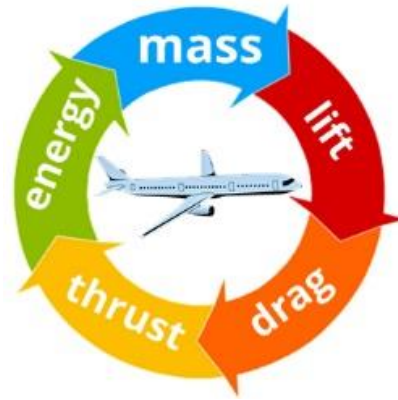
Figure 9: Improvements of aircraft leading to a lower energy consumption enhance each other. Mass and thus weight reductions have a positive effect on lift, drag, thrust and energy consumption, leading to less fuel to start with, leading to less mass, which results in a “snow-ball” effect.
