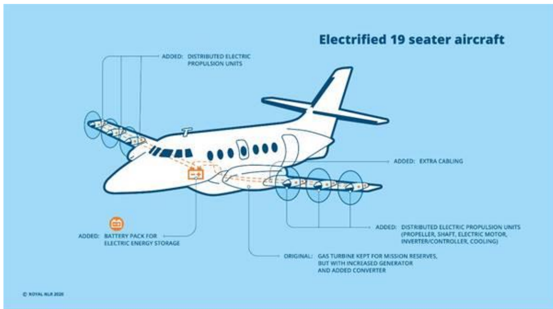
Figure 21: Distributed propulsion applied to a 19 seater electric aircraft (NLR).
