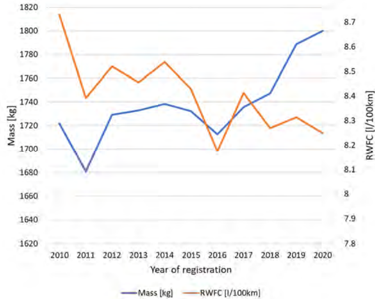
Figure 3-3: Trend of average vehicle mass and real-world fuel consumption per registration year for diesel vans (excl. plug-in hybrids).
