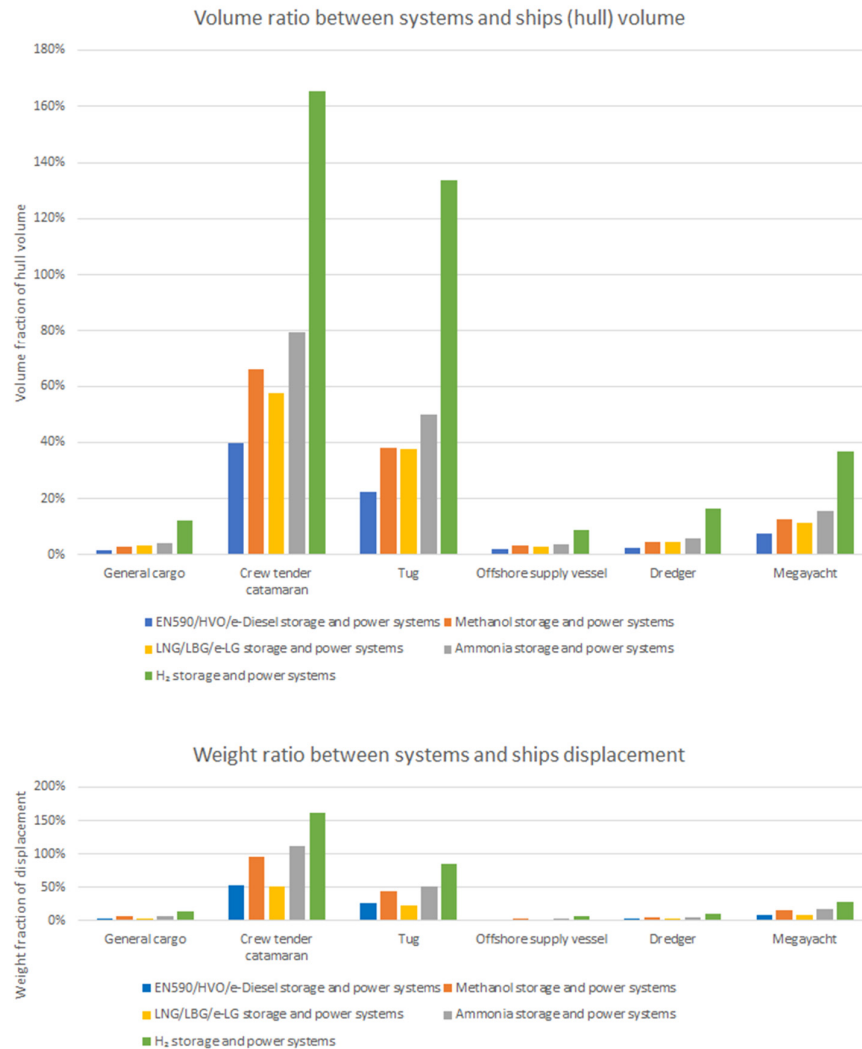
Figure 2: Volume (top) and weight (bottom) ratio (PPE-system compared to entire ship).
