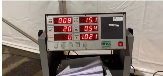
Inspection of a ten-year-old Euro 4 Hyundai for Ghana with functioning catalytic converter
