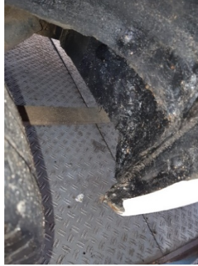
Ford Transit from 2006 for Tema, Ghana: auxiliary beam chassis incorrectly repaired, sills incorrectly welded
