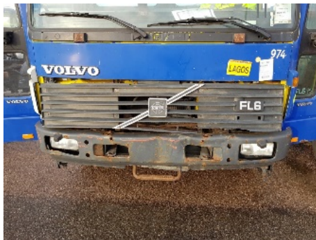
A Volvo from 2000, for Nigeria with many deficiencies: VIN unreadable, lights and battery removed, exhaust system incomplete, bumper missing, fuel tank missing, air tanks hanging loose, smooth tires
