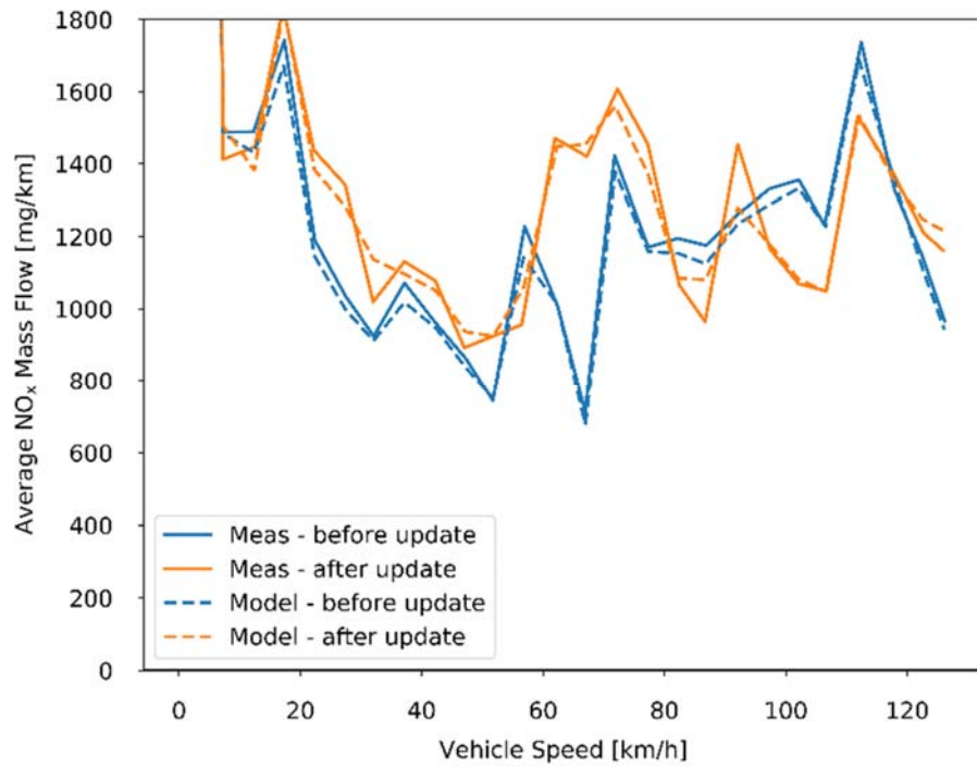
Figure 7.2: The velocity dependent emission data of the Audi A4, uncorrected, and corrected for test conditions and test execution.
