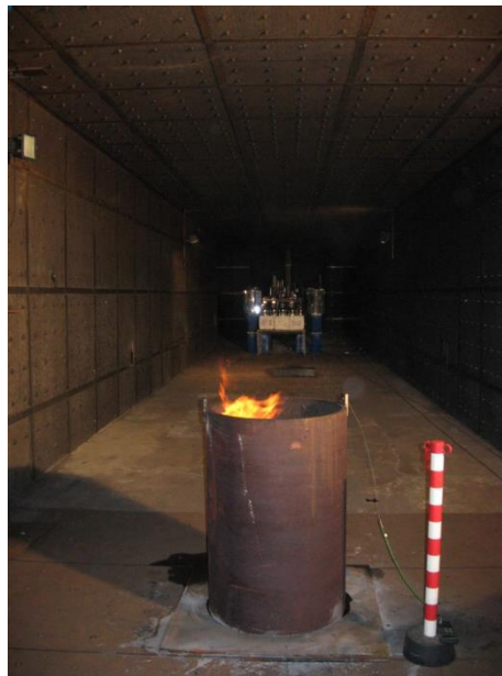
Figure 3 Initial test set up with sampling height at 1.8 m.
