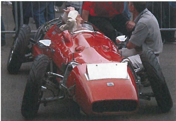
Figure 9 Wheel alignment has a major impact on the roadholding characteristics of the car and on tyre abrasion. Photo: Milliken MX1 Camber Car 1960 driven by Bill Milliken (Brian Snelson).
