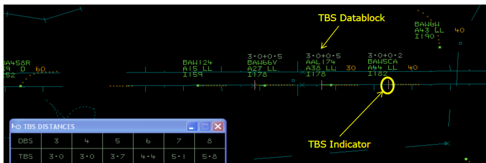
Figure 15: Indicators on the Radar screen point at the optimized aircraft positions when applying Time Based Separation. This concept can also be used for other types of separation and also for example when merging streams in the TMA. Source: [NATS Lockheed, 14].
