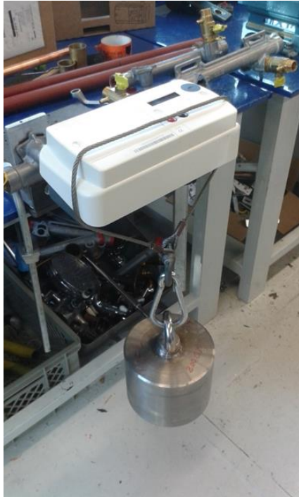
Left: bending test; right leak tightness test.
