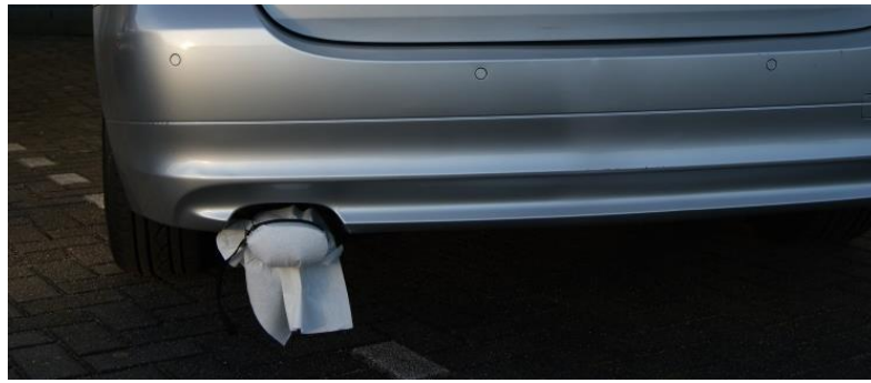
Figure 16 In the tissue filter test, a tissue was attached to the end of the exhaust pipe after which the engine was let running at idle speed for three minutes. Cars showing elevated emissions in previous tests were selected for the TFT.
