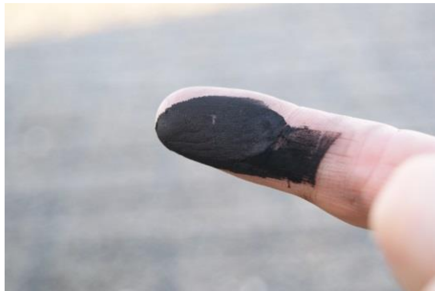
Figure 8 Example of two tailpipe swipe tests resulting in a deep black finger, scoring 3.
