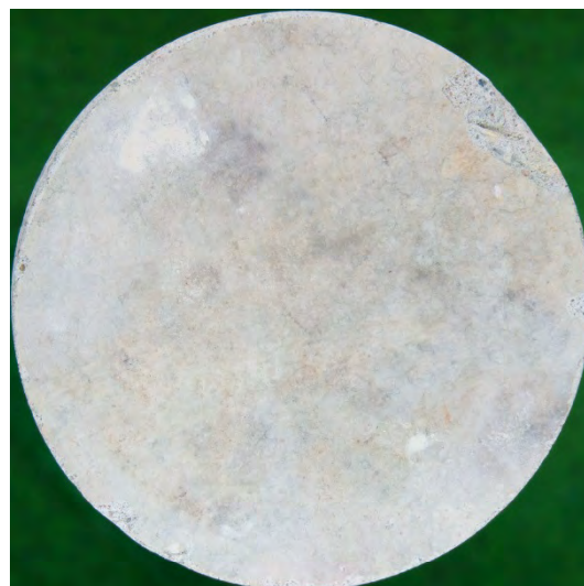
Figure 15: Photo of the surface of core M68-9. The surface is plane and smooth.
