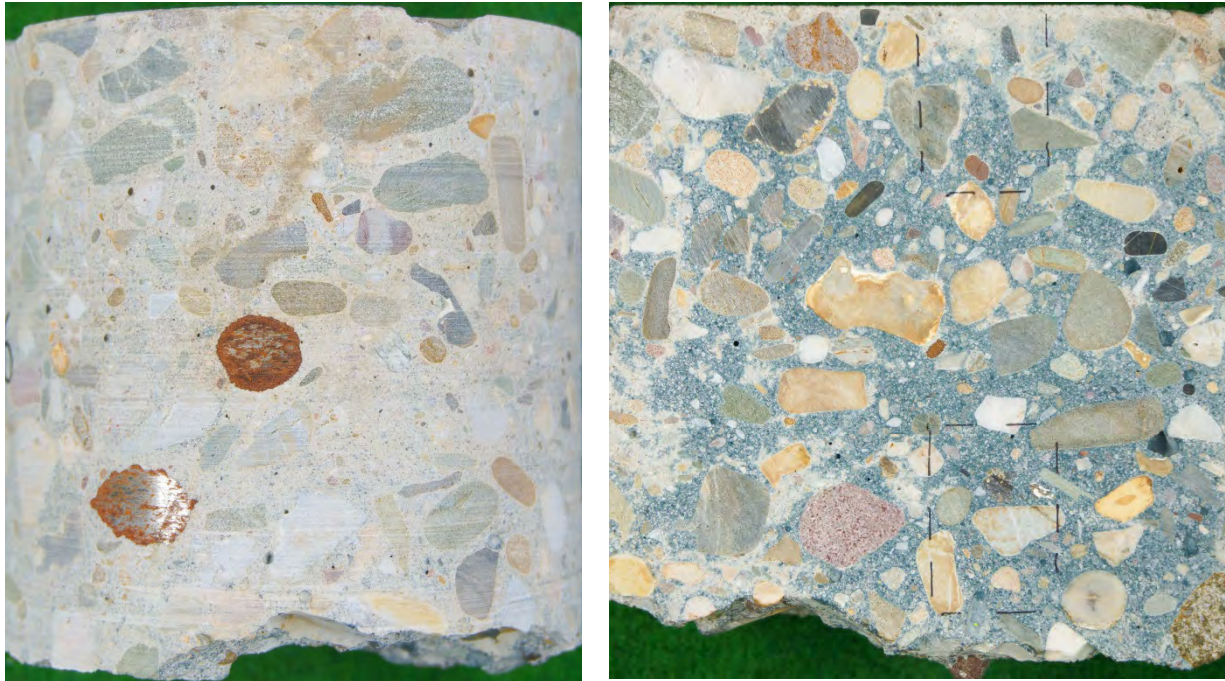
Figure 8: Photos of core M66-K9 with the surface upwards. The left photo shows the full core as received; the right photo shows the axial section of the (non-impregnated) core seen in white light. Positions of thin sections are marked with black dotted lines.
