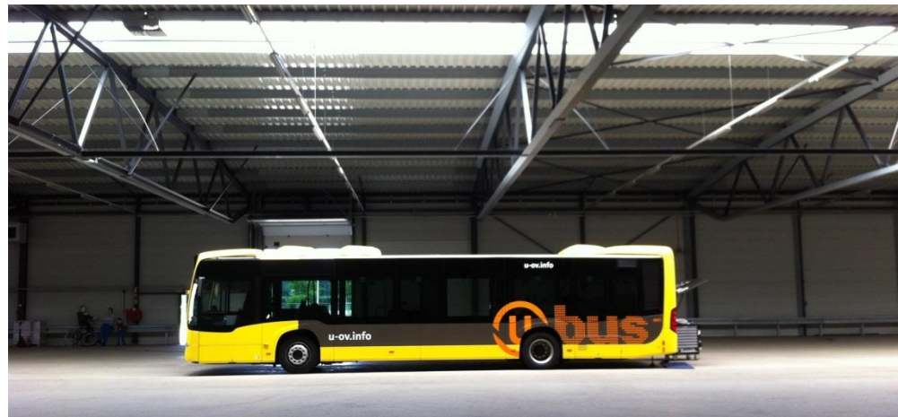
Figure 1: The test vehicle: a Euro-VI 12-meter Mercedes Citaro, kindly provided by Qbuzz.
