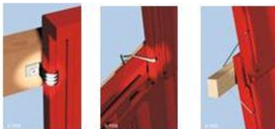
Figure 29 Examples of mechanical tile fasteners.
