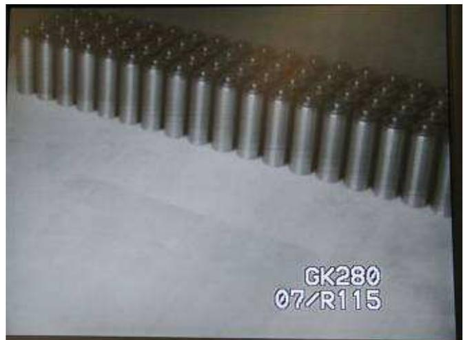
Figure 1.7 Non-heat producing waste storage
