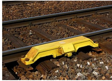
Image 17 - PZB Track Balise
