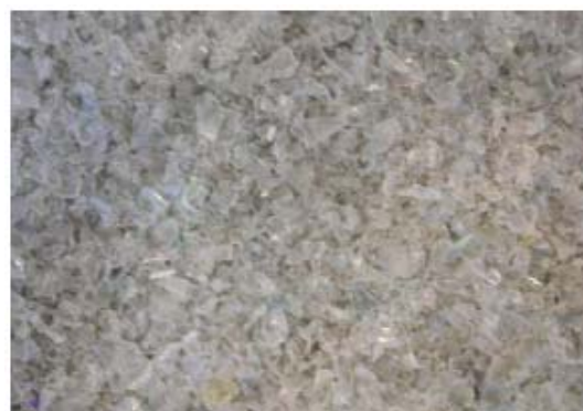
2 nd pass Clear PET from S+S trial (98.76% purity)
