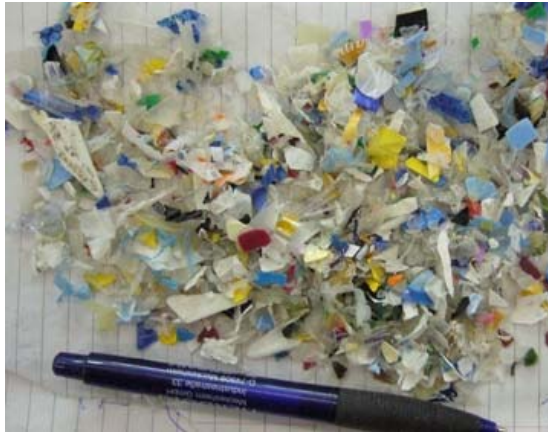
Dry cleaned rigid flaked PP from NIR sorting
