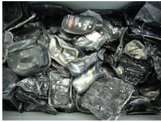
Hand sorted black plastic from residue output
