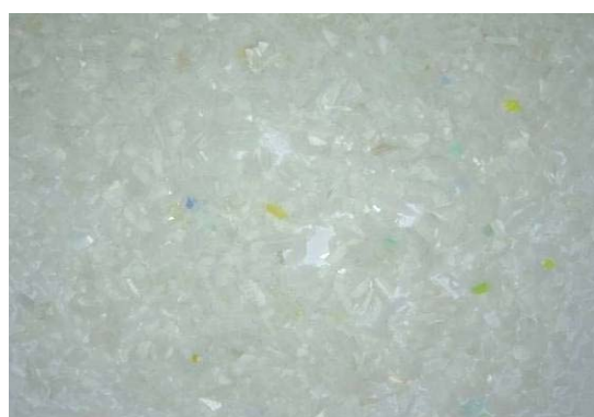
3 rd pass clear PO flake from SEA Srl trial (99% purity)
