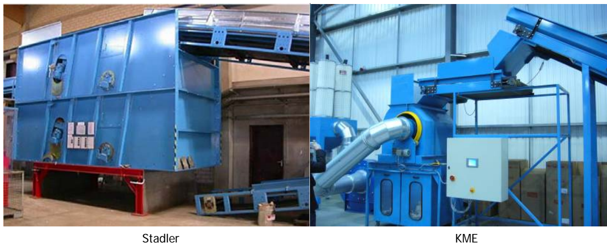
Figure 17 Stadler STT2000 and KME Air Drum Separator
