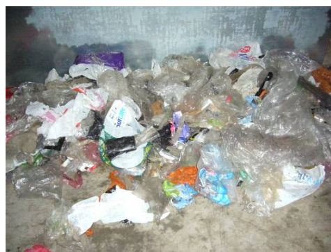
Figure 4 Sorted film fraction
